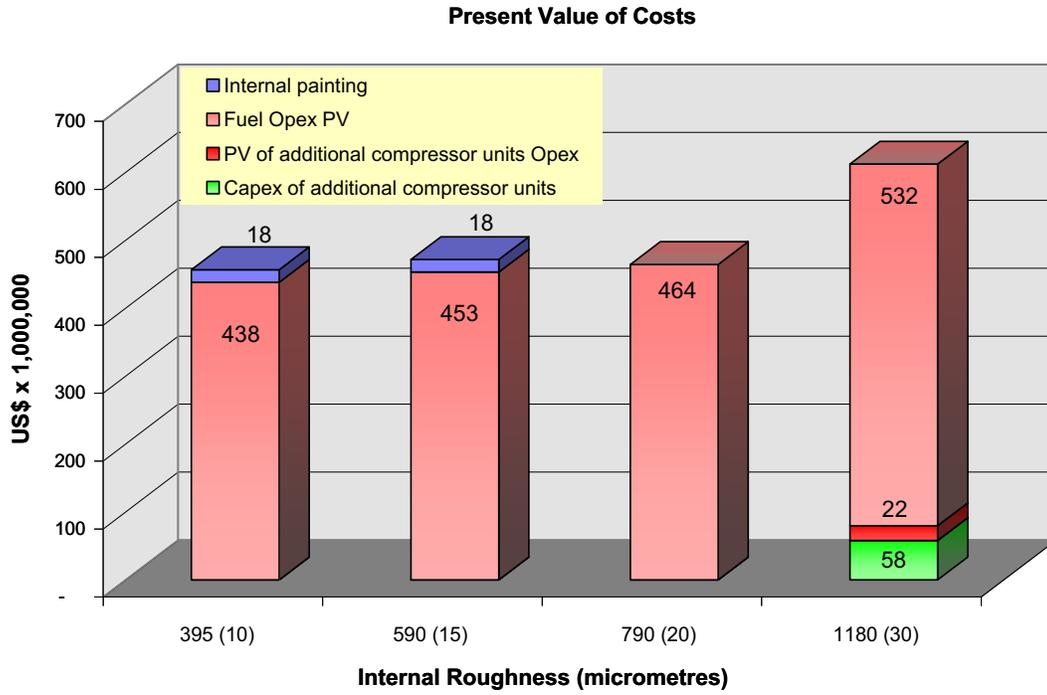
Figure 3 – Present Value of OPEX and CAPEX
