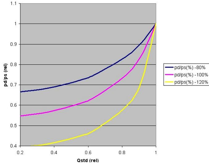
Figure 1 - Pipeline characteristics for different pipeline resistance for nominal loss coefficient, 80% of nominal loss coefficient and 120% of nominal loss coefficient. (Lubomirsky et al, 2010).
